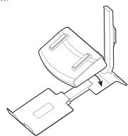
4 Attach the Notebook Holder's VESA fitting to the monitor arm ball joint connector by sliding the VESA fitting onto the ball joint connector and snapping it into place.
