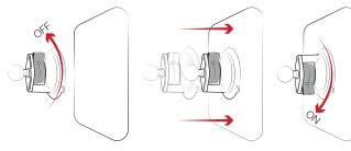
RAM® Twist-Lock™ Suction Cups are only compatible with smooth, non-porous surfaces (no rough or textured surfaces). Clean surface thoroughly before applying suction. When left unattended in extreme temperatures, it is recommended to remove and stow suction cups. Suction cups are considered a general wear item and are not covered under any warranty.
